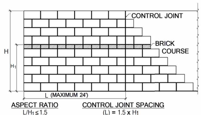
**Figure 2. Control Joint Spacing**
