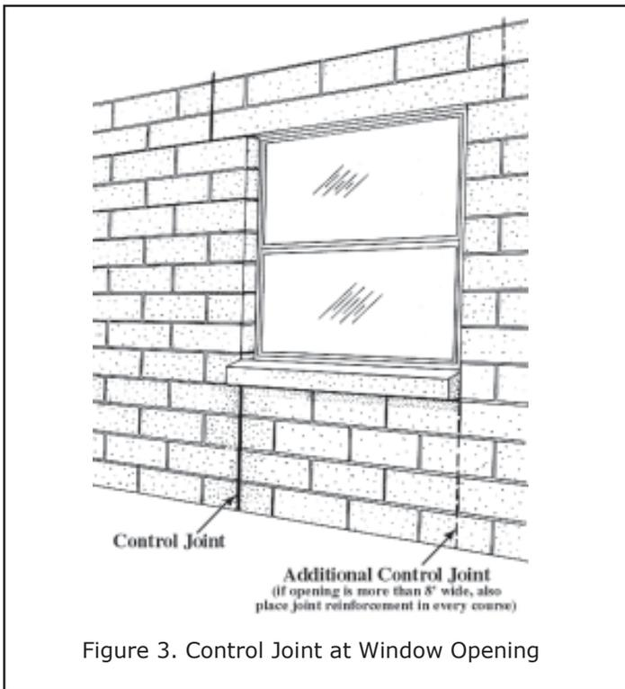
Figure 3. Control Joint at Window Opening
