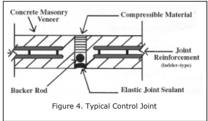
Figure 4. Typical Control Joint
