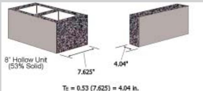
Concrete masonry units (CMU) are commonly manufactured with a combination or blend of aggregate types. The International Building Code covers this condition by reference to standard TMS 216 (ref. 5). The minimum equivalent thickness value required for a desired fire rating can be determined by interpolating between requirements for different aggregate types in proportion to the percentage by volume of each aggregate used in manufacture.
